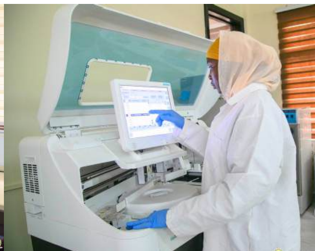
Figure 4: A biomedical scientist using a Roche Cobas analyzer for thyroid function analysis
