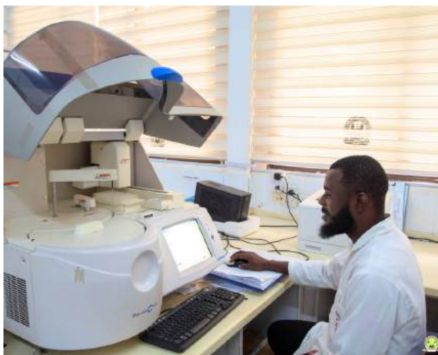
Figure 3: A medical laboratory technician is using the chemistry auto analyzer for organ function analysis in study participants
